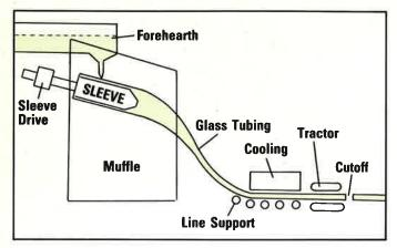
In the Danner Process, glass tubing is made by "flowing" a continuous stream of molten glass of a precise viscosity onto the surface of a downwardly sloping, rotating hollow mandrel (sleeve) where it levels or "marvels" to form a thick cylinder of molten glass. Air is blown through the center of the sleeve to maintain the hollow interior of the tubing. The combination of glass quantity, glass temperature, speed and air determine the size of the tubing.
