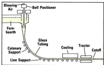
The MDD process involves "flowing" molten glass through an annular orifice in the bottom of a bowl and blowing air through the interior of the resulting tubing. Glass temperature, drawing speed and the force of the air are all tightly controlled to produce a continuous length of tubing to precise diameters and wall sections.
